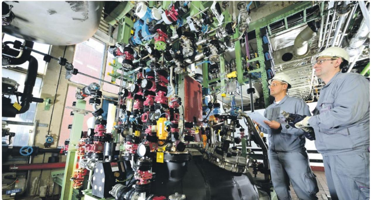
of various devices to form new combinations — as required by the synthesis process — can be carried out efficiently. In the Central Organics Pilot Plant (Zentrales Technikum Organisch, ZeTO) alone, there are twelve such interfaces. They enable material flow by bringing together pipe connections of numerous apparatuses. Bridged with flexible hoses, almost any circuitry can be realized easily and quickly.
