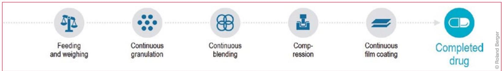
Fig. 1: Example of a schematic continuous production process.
