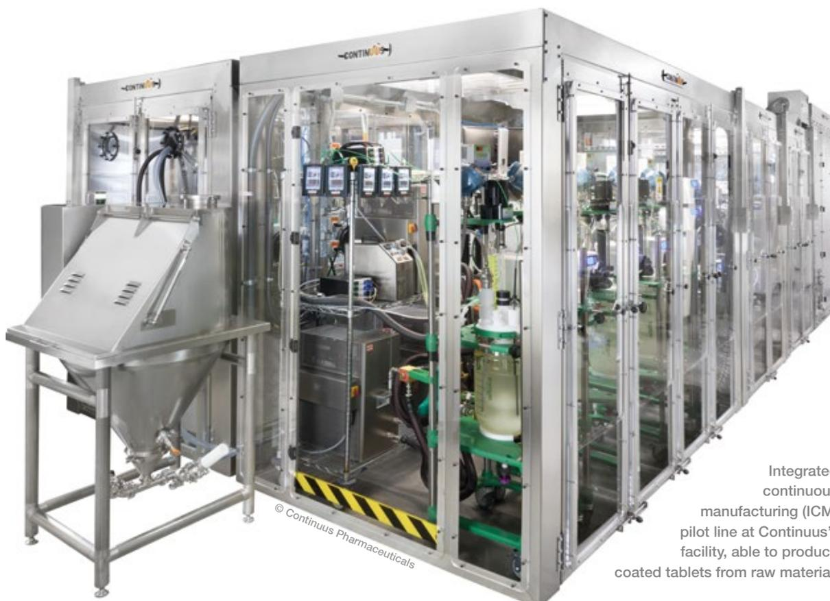
Integrated continuous manufacturing (ICM) pilot line at Continuous's facility, able to produce coated tablets from raw material.
