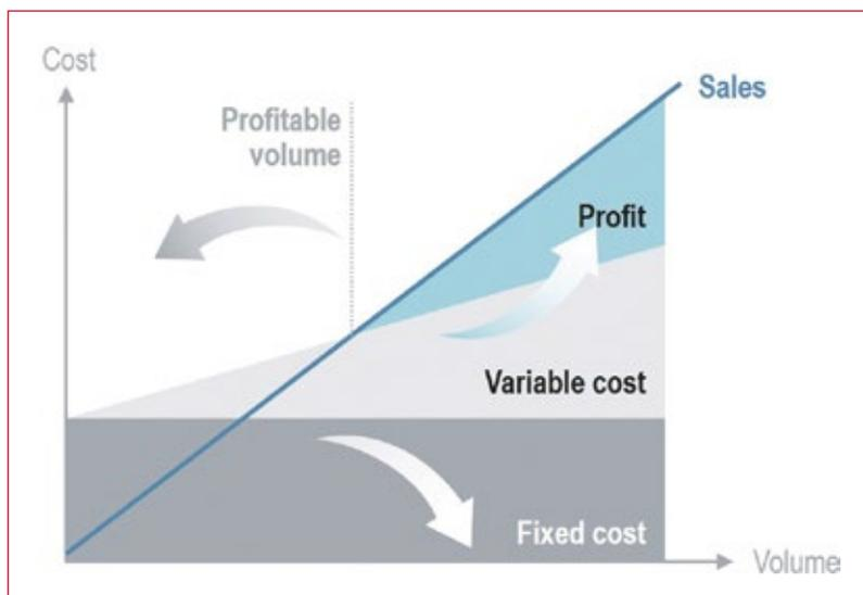
Fig. 2: Continuous production can reduce fix and variable costs and increase product profitability.
