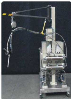
Silicone dosing machine integrated with Sitrans F C Mass 2100 Coriolis flowmeters
