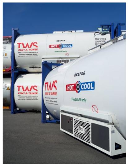
Chemical or foodstuff industry: Special reefer tank containers allow the liquid products to be cooled to -20 °C and heated up to 50 to 80 °C, depending on the
