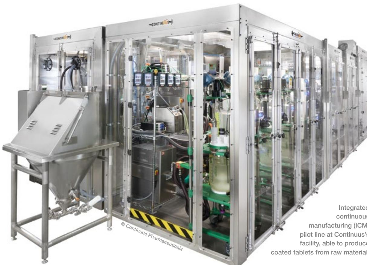
Integrated continuous manufacturing (ICM) pilot line at Continuous's facility, able to produce coated tablets from raw material.
