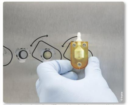
Single-use flow cell with silicon ATR crystal. It easily click-mounts to Monipa.
