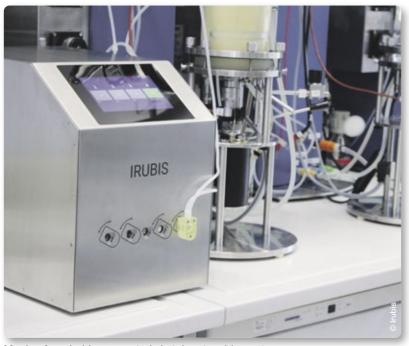
Monipa from Irubis connected via tubes to a bioreactor
