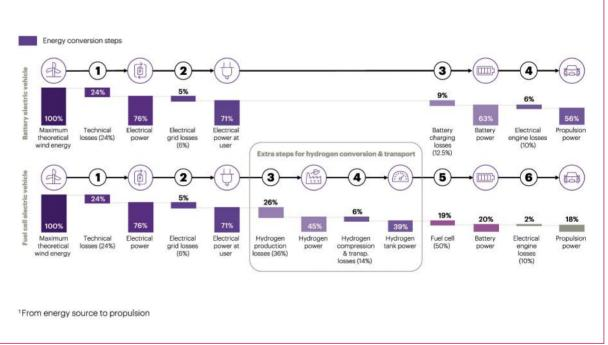
Fig. 2: Comparison of well-to-wheel efficiency from energy source to propulsion.
