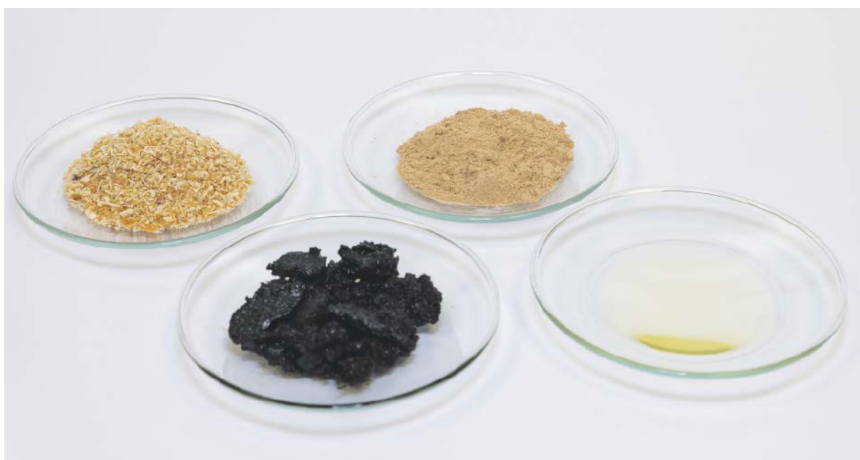
Sonichem's patented breakthrough approach converts sawdust, the biomass by-product from forestry operations, into high-quality lignin which can then serve as the basis for bio-based platform chemicals.
