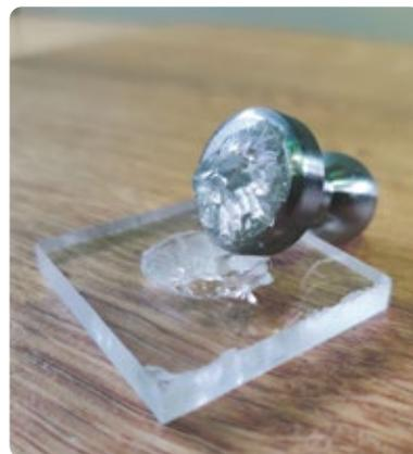
The RadiBond technology combines chemically different materials. The result is plastic-breaking strength even for challenging plastics.
