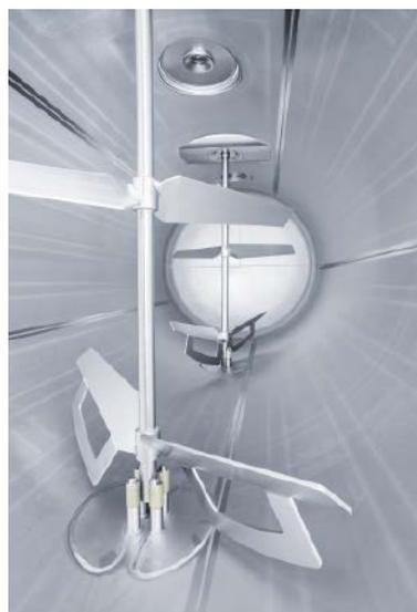
The adaptability of the tank container is mainly due to its technical equipment, e.g. vertically installed agitators with two blades that are guided through Teflon sleeves.
