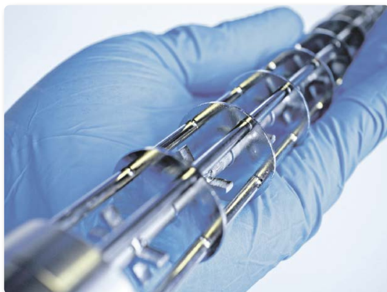
Fig. 2: The insert of the SABRe highlighting the innovative baffles and stirrer configuration.
