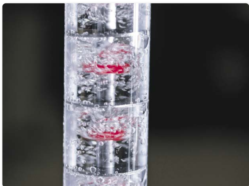
Fig. 1: Mixing in action in the SABRe highlighting the capability of the reactor.
