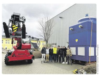
A modular container that houses Greenlyte's DAC technology, which can extract CO<sub>2</sub> from ambient air and turn it into green hydrocarbons.
