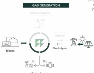
Reverion's plants have a reversible operation mode: They can electrochemically convert biogas or hydrogen into electricity and can also produce green hydrogen or methane from electricity (power-to-gas), both with highest electrical efficiencies of 80%.
